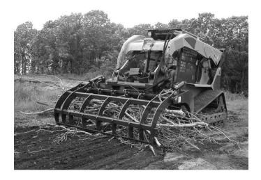
4. To back rake, fully open the grapple, tilt the loader coupler forward until the grapple teeth contact the ground, lower the boom to apply down pressure, and slowly drive backward to rake material.
