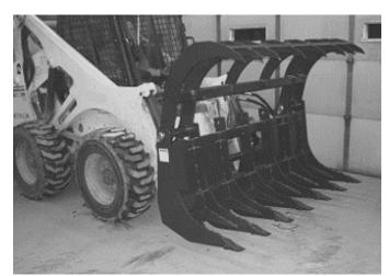
3. Activate the loader's auxiliary hydraulics to open and close the grapple in order to pick up and move debris/objects.
